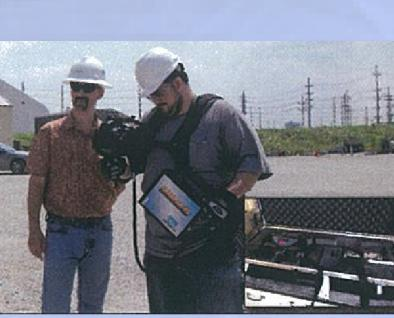
A Heath Remote Methane Leak Detector (RMLD) was modified to detect carbon-dioxide level by replacing the laser module, and the infrared detector with devices operating at 2.0 µm.
